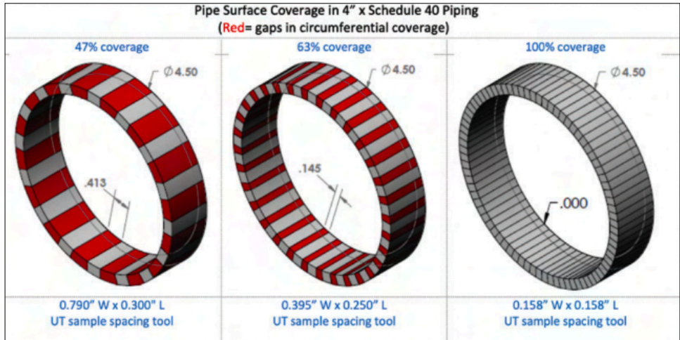
Figure 9. UT sample spacing comparison of pipe cross-section.
